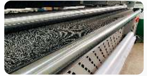
Strengthful chrome plated shaft, to secure the feeding of media straight and flat, for better print output.
