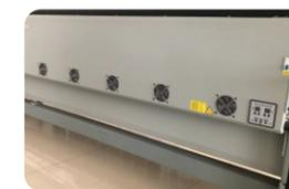
2 individually controlled powerful dryer system, to start and stop automatically when a job starts or stops.
