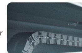
IGUS caterpillar chain, durable to move back and forth silently with cables and tubes well protected inside.
